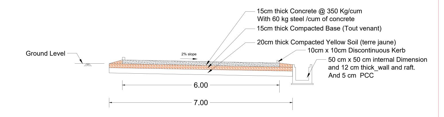
**Cross section of Road and Drain**
